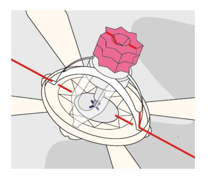
To be correctly positioned, one of the arches of SeeStar® shall be placed in the plane and aligned with the laser line produced by the CT equipment. To help the placement, there are notches in the baseplate that shall match with the laser line.
