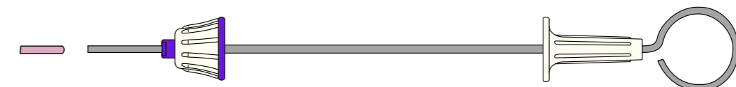
Ejection of sample from biopsy cannula using sample ejector pin and sample ejector guide
